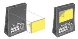
Figure 7. Wall-mount the Internet adapter
